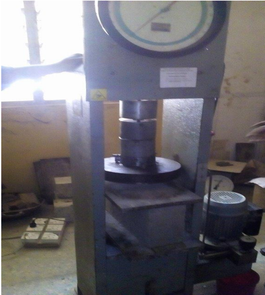
Fig 2. A sandcrete block subjected to compressive loading in a universal testing machine
