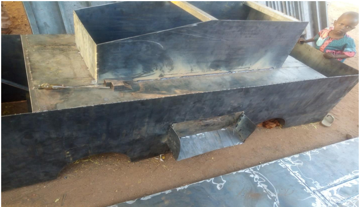
Plate 9: A fabricated incinerator showing a combustion chamber and outlet of ashes of a burnt materials/waste
