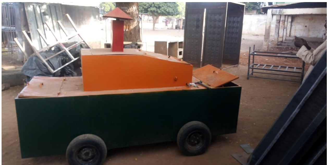
Plate 11: A fabricated mobile incinerator showing three units (chimney, combustion chamber and the gas and ignition unit) coupled with wheel and axle
