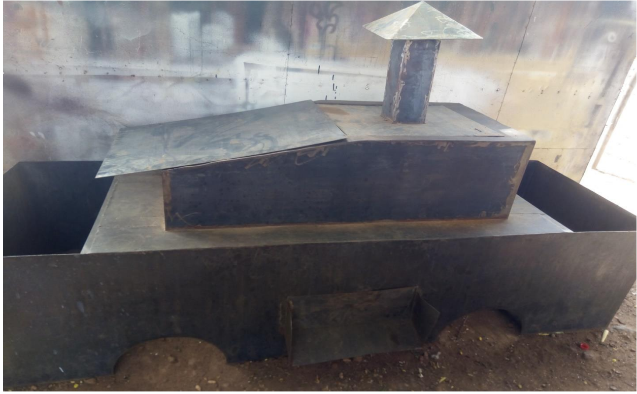
Plate 10: A fabricated incinerator incorporated with a chimney before wheel and axle were coupled
