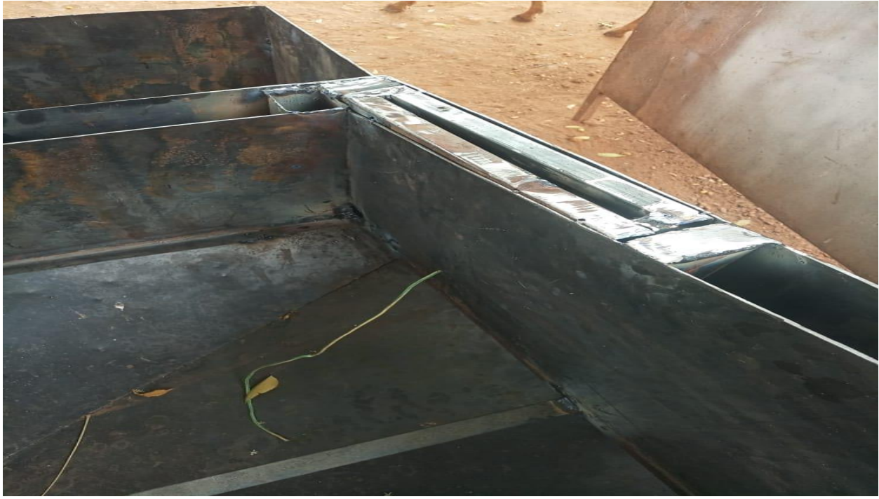
Plate 4: A fabricated incinerator the showing position of filling with clay for lagging
