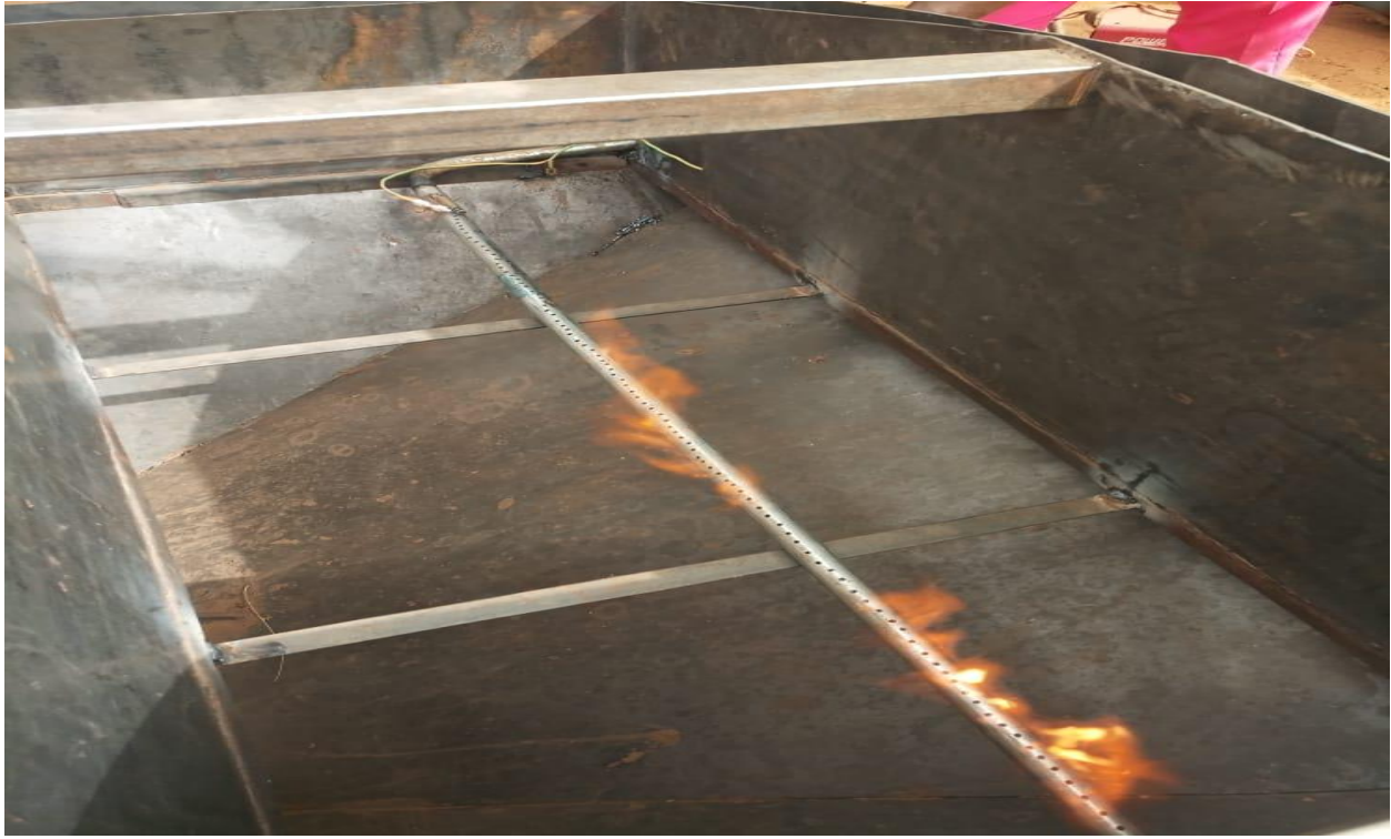
Plate 8: Provision and ignition of heating element showing fire flame (as a burner) to the Incinerator
