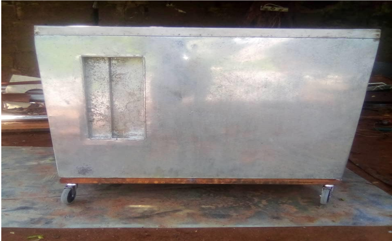
Plate16: Hydraulic bench showing point where Single phase breaker is to be fixed.
