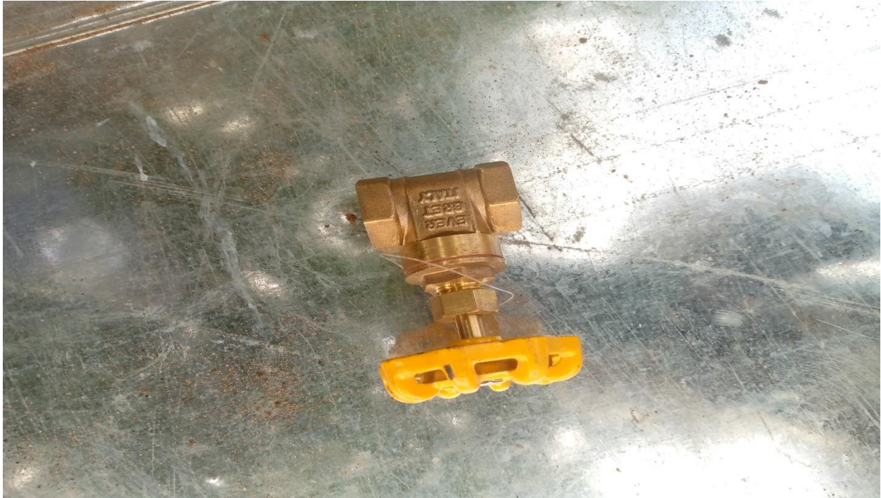
Plate10: Half inch ON/OFF Gate Valve used in the hydraulic bench for pumping
