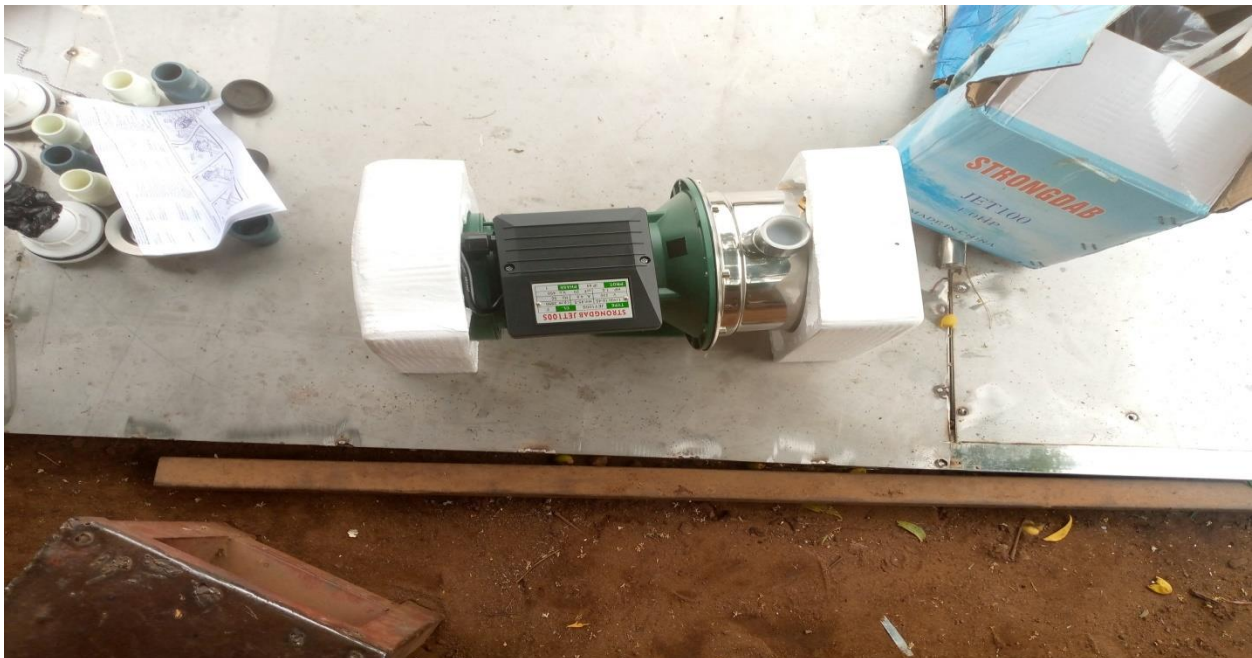
Plate9: 1hp Centrifugal pump that draws water from sump tank and supplies it for performing experiment
