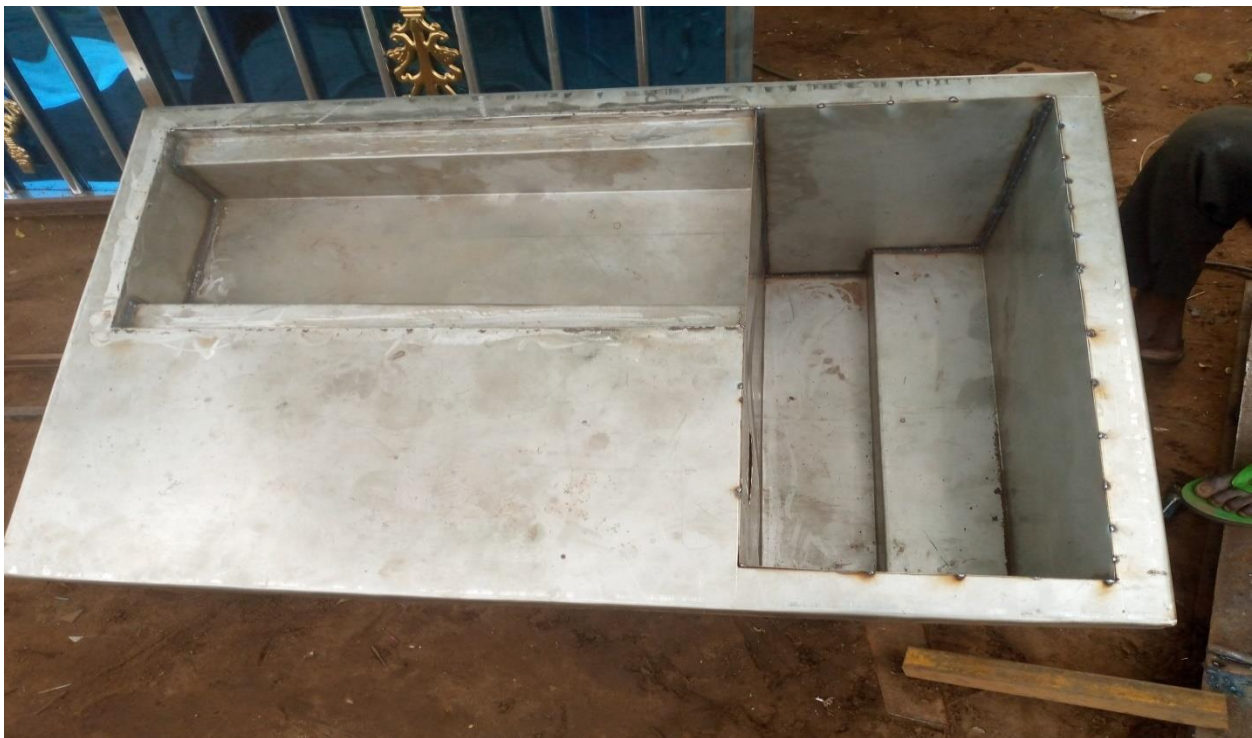
Plate7: View of a Welded connected top of the hydraulic bench
