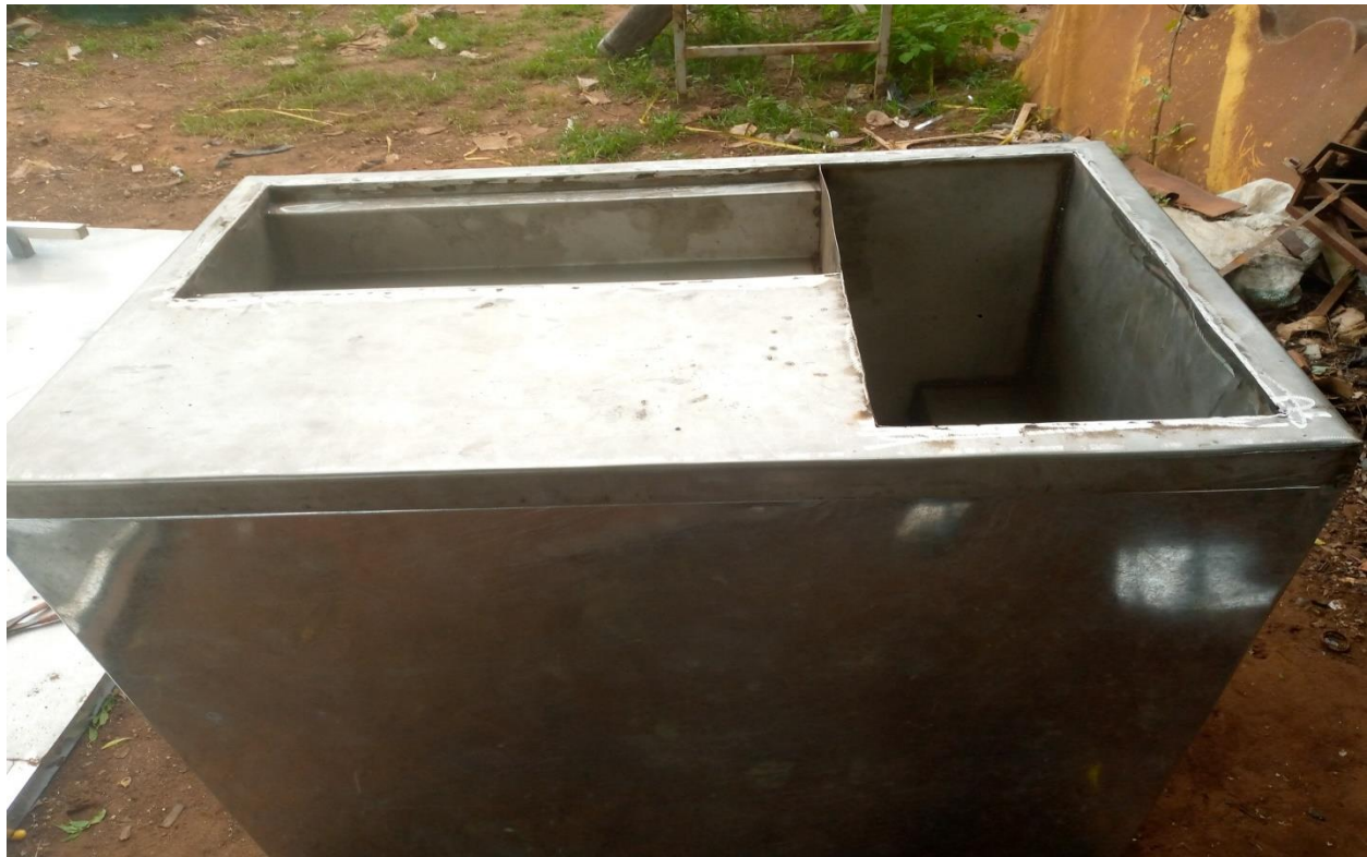
Plate13: View of the fabricated Hydraulic bench before filing and painting
