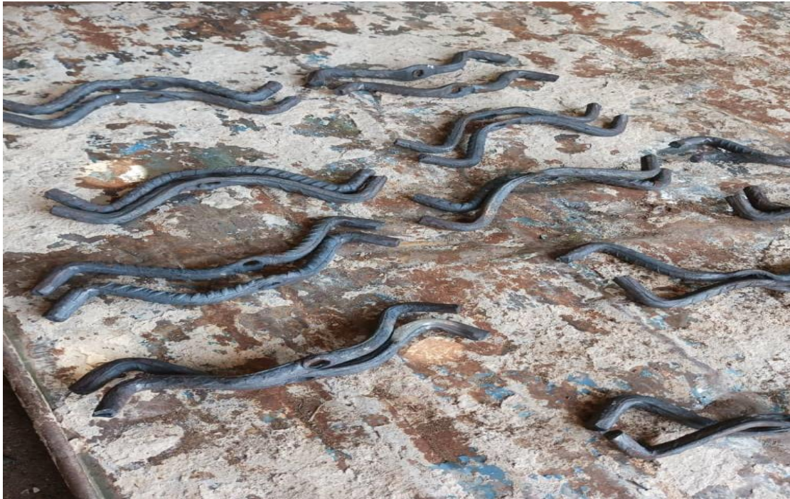
Plate 1: Handles constructed to hold the mold during the molding of concrete cube.
