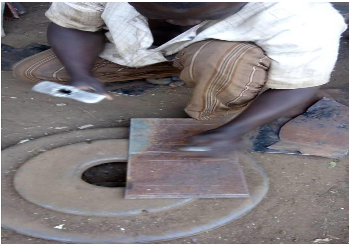
Plate 3: Cutting of slates.
