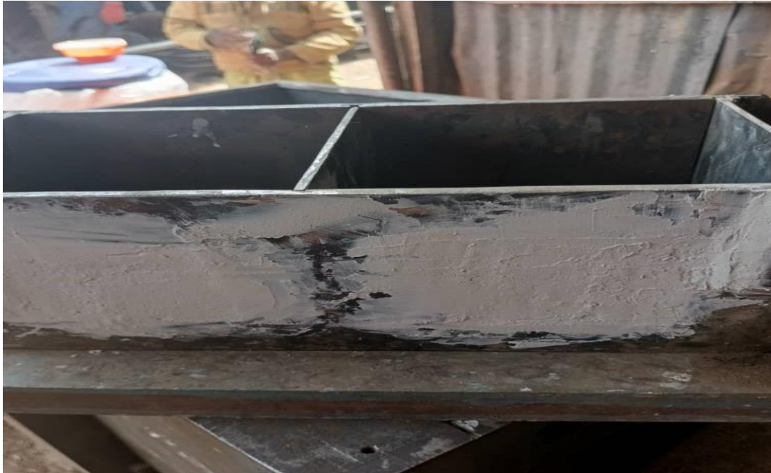
Plate 6: A dual-cell metal concrete mold ready for smoothing after body filling.
