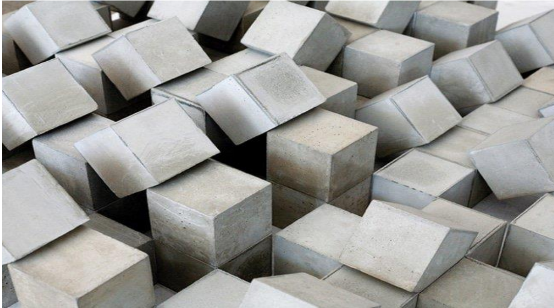
Figure: Specimen of concrete cubes
