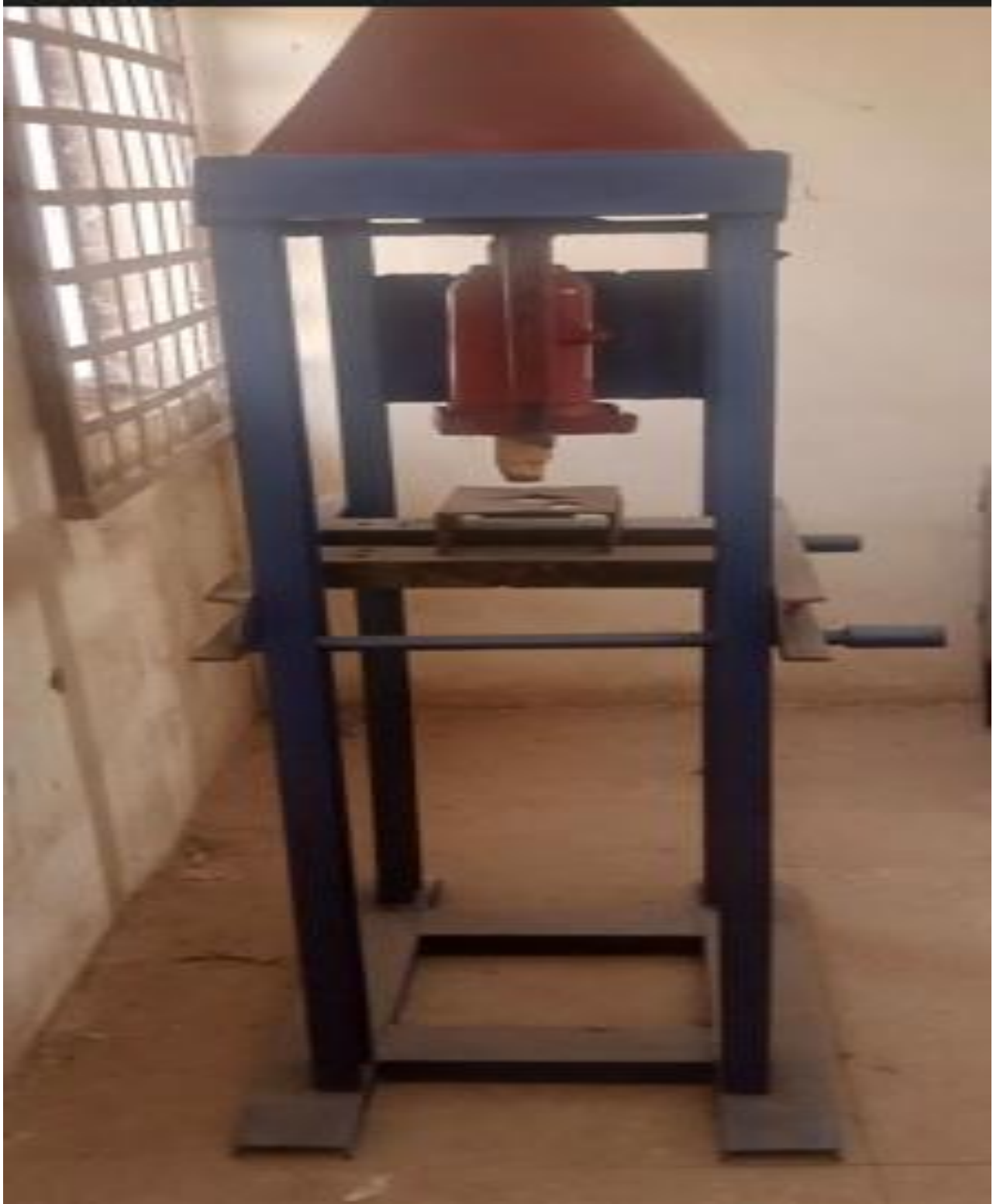
Side view of the hudraulic pressing machine
