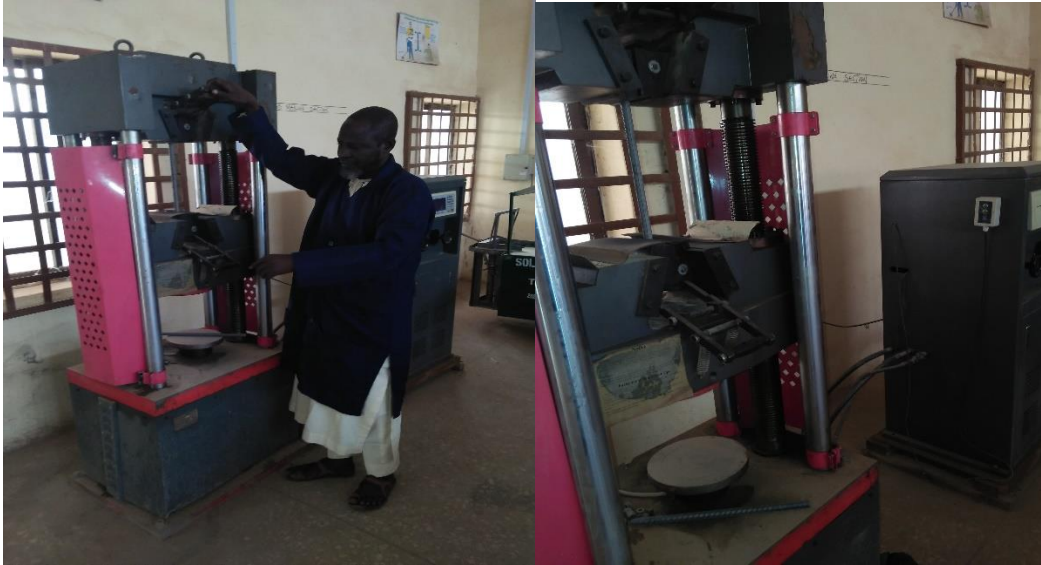
Plate 1: Working with the Universal Steel Tensile Testing Machine
