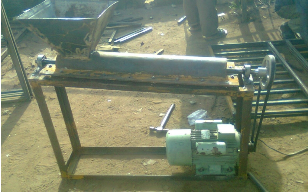
Plate 3.1. A Pictorial View of the fabricated Shea Nut Decorticator
